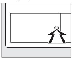
Press the round, indented area on the heat exchanger access panel to open it.
